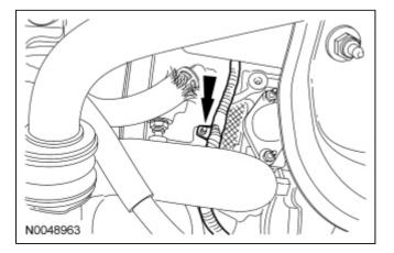
23. Position the A/C compressor, bolt and install the 3 nuts.Tighten to 25 Nm (18 lb-ft).
