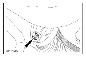
6. Install the LH radio interference capacitor and nut onto the engine front cover stud bolt.Tighten to 25 Nm (18 lb-ft).
