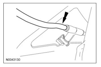
37. Install the hood insulation pin-type retainer and attach the 2 windshield washer hose retainers.
