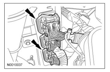
11. Connect the generator jumper harness electrical connector.
