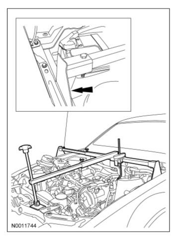
4. Remove the Engine Lifting Bracket.
