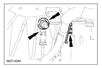
26. Attach the 2 pin-type retainers.
