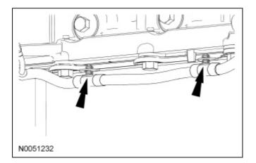
27. Connect the coolant hose to the oil filter adapter.
