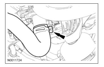
28. Connect the A/C pressure transducer electrical connector.
