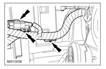
10. Connect the upper and lower PCM electrical connectors.
