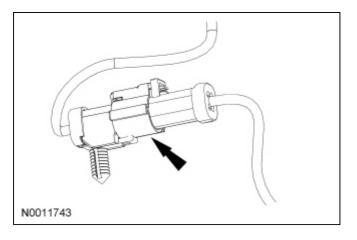
16. Connect the RH Heated Oxygen Sensor (HO2S) electrical connector.
